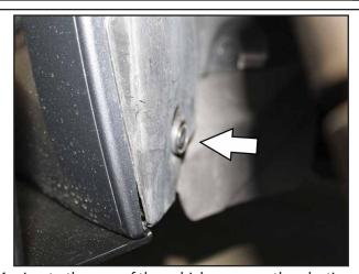
Moving to the rear of the vehicle, remove the plastic fastener directly in front of the rear wheel in the wheel well. Removing all these fasteners aid in gaining access behind the rocker panel to install the hardware later.
