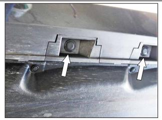
Remove the plastic fasteners along the underside of the rocker panel using a panel removal tool or flat head screwdriver.
