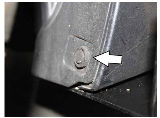
Remove the plastic fastener located directly behind the front wheel in the wheel well.
