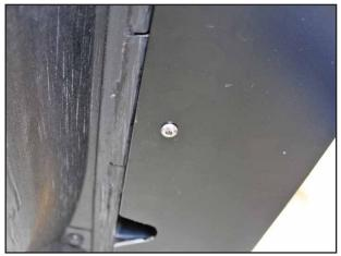
Fasten the splitter to the rocker panel via (1) 1/4"-20 Socket Buttonhead Bolt, (1) 1/4" USS Flat Washer, (1) 1/4" Split Lock Washer, and (1) 1/4"-20 Hex Nut.
