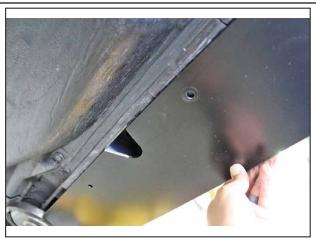
Hold the splitter up against the body and line up the large holes with the holes where the plastic fasteners came from. Also, align the rear cutouts with their respective edges toward the rear of the rocker panel.
