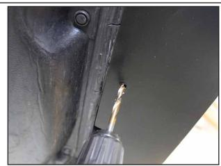
Mark and drill out the mounting holes along the underside of the rocker panel using the splitter as a template.
