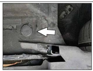
Staying behind the front wheel, there is another plastic fastener directly under the rocker panel - remove this as well.
