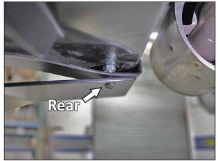
Hold up the splitter against the bumper, aligning the mounting holes with the holes in the bumper. Insert (1) 1/4"-20 Socket buttonhead through the bottom and fasten with (1) 1/4" Flat Washer, (1) 1/4" Split Lock Washer, and (1) 1/4"-20 Hex Nut on the inside of the bumper.
