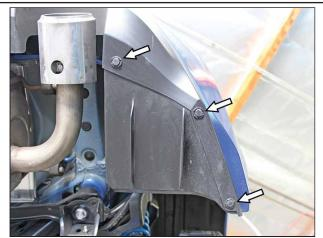
Locate and remove the plastic fasteners at the bottom of the rear bumper on each side (driver and passenger).
