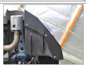
Tighten down the hardware using a 5/32" Allen Key and 7/16" Wrench. Repeat for driverside.
