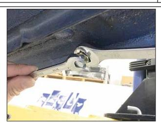
Hold the riv nut collar still with a 5/8" wrench and tighten the riv nut tool with a 7/16" socket/wrench. Tighten the tool until the riv nut is completely compressed (one way to check is it no longer spins freely in the hole). Repeat for all mounting holes.
