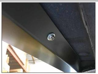
Attach each side splitter to the car using (1) 1/4"-20 Buttonhead Bolt, Lock Washer, and Washer for each hole. Tighten all hardware.
