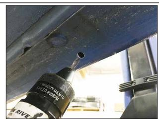
For each hole, drill out a pilot hole (1/8" or similar size) first, then proceed to increase the drill hole size until you reach the 25/64" hole required to fit the riv nut.
