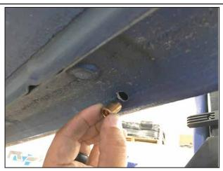
Insert the riv nut into the hole then install the riv nut tool onto the riv nut.
