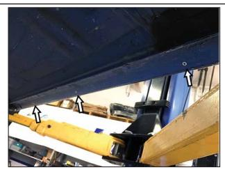
Hold side splitter against the body to mark centerholes for drilling.
