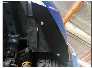
Insert (1) 5/16"-18 x1" Socket Buttonhead, (1) 5/16" Washer, (1) 5/16" Lock Washer, and (1) 5/16"-18 Nut into each mounting hole for the rear splitter (center hole not required for use).
