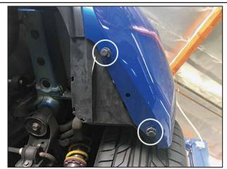
Locate and remove the clips in the rear bumper. These will become the mounting holes for the rear splitter.
