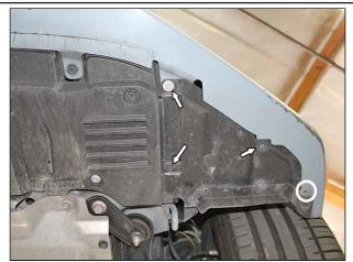
Locate and unfasten the factory clips on the fog light splash guards - this will aid in installation. Locate the farthest right hole (circled above) and fasten the corner of the driver-side splitter loosely to hold it in place. Repeat on the passenger side.
