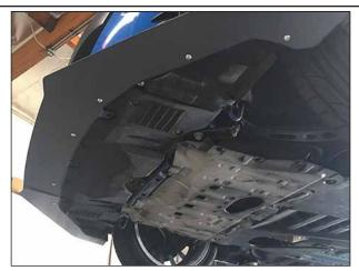
Insert (1) 5/16"-18 x1" Socket Buttonhead, (1) 5/16" Washer, (1) 5/16" Lock Washer, and (1) 5/16"-18 Nut into each mounting hole. Loosely fasten hardware initially, until all bolts are in. Make sure the splitters are aligned and then tighten them down.
