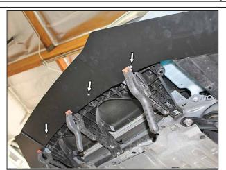
Next place the center splitter piece inbetween both ends and clamp/hold the splitter pieces in place as you mark the mounting holes for drilling. Note the center piece rests on top of both end pieces. Drill holes out to 5/16 inch.
