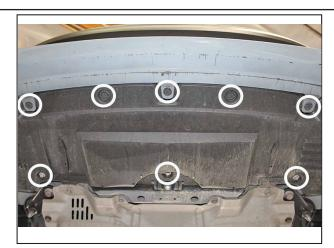
Remove factory splash guard by unfastening factory clips holding it in place.
