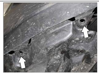
Remove the necessary clips from the foglight splash guard, which is located in front of each front wheel and below the front bumper. This will allow access to the foglight area.
