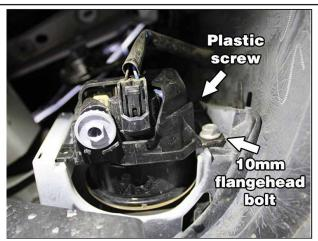
Remove the plastic screw clip with a flathead screwdriver. Then, remove the 10mm flangehead bolt with a 10mm socket. This will free up the foglight and it should slip out. Don't forget to unplug the light from its harness.
