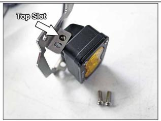
Assemble Baja Designs light and light conversion bracket using the included small screws in the Baja Designs light package. Mount the light to the top holes on the bracket like shown in the picture.
