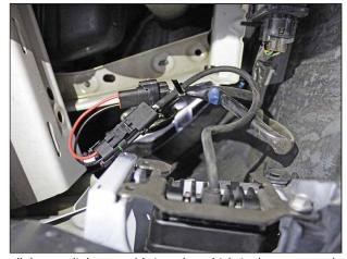
Install the new light assembly into the vehicle in the reverse order of removing the factory foglight. Reuse the factory hardware. Plug in the wiring adapter harness (if you have it) into the light and then into the vehicle harness. Fasten the harness to a secure location.
