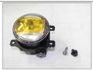
Here is what you should have removed in the previous step. Retain the hardware for install of the new light assembly.
