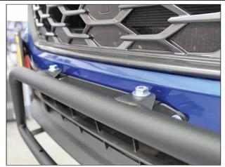
Mount the light bar to the license plate bracket with (1) 3/8"-16 x1.5" Hex Bolts, (2) 3/8" Flat Washers, (1) 3/8" Split Lock Washer, and (1) 3/8" Hex Nut on each hole.
