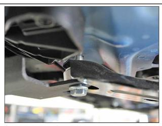
Insert the M8x40mm flangehead bolt through the bracket and into the chassis. Tighten down.
