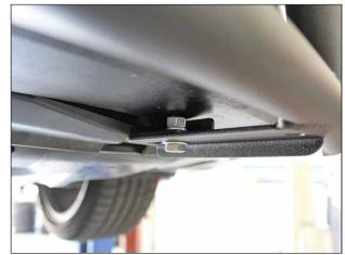
Mount the light bar to the lower brackets using (1) 3/8"-16x 3/4" Hex Bolt, (2) 3/8" Flat Washers, (1) 3/8" Split Lock Washer, and (1) 3/8" Hex Nut on each hole.
