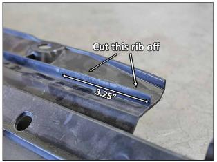
Flip the splash guard over (so it's as if you're viewing it from inside the engine bay). Adjacent to the cut-out just made, trim the rib shown (3.25" long). Use the utility knife again.
