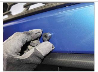
Insert the included M6 well nuts into the holes.
