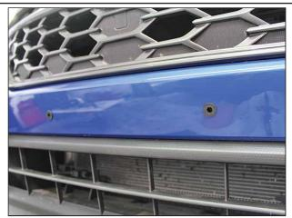
Bumper cover with well nuts installed.
