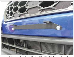
License plate bracket installed with (2) M6 flange head bolts
