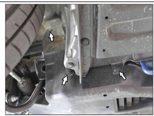
Remove these fasteners in both wheel wells.
