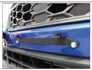
Next place the (2) cylindrical nylon spacers on top of the license plate mounting flanges.
