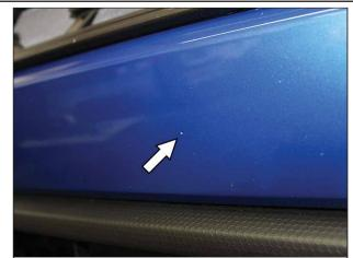
Use the factory front license plate mounting holes to mount the License Plate Bracket. If bumper does not have these holes, locate the factory indentations on the bumper cover and drill them out to 1/2".
