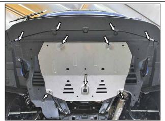
Remove the engine splash guard by removing the fasteners shown above.
