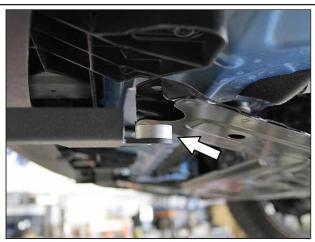
Insert the 1/2" cylindrical aluminum spacer between the right mounting hole on the bracket and the vehicle chassis.
