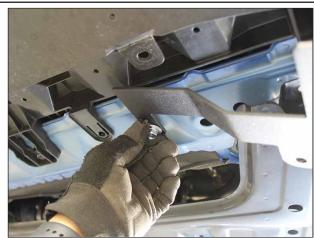
Install the bracket in the orientation shown. Use the previously removed 12mm-head bolt to loosely fasten it in place on the mounting hole to the left. Tighten it just a few threads.
