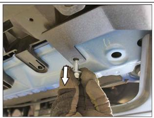
Remove the M8 bolt inserted in step 6. This hole will be secured at a later step 17.
