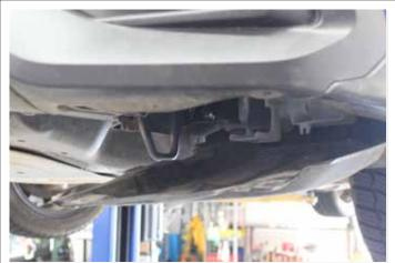
Remove splash guard. Remove fender plastic rivets to allow access behind the foglights.
