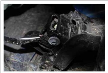
Unplug the foglight harness and undo the plastic screw and Phillips screw shown above (keep for later).
