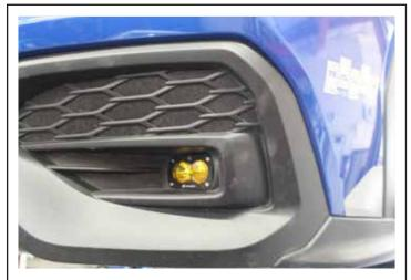
Reinstall fender cover, splash guard, and front bumper cover (if removed) using factory plastic clips. *Pictured: Completed Assembly.*
