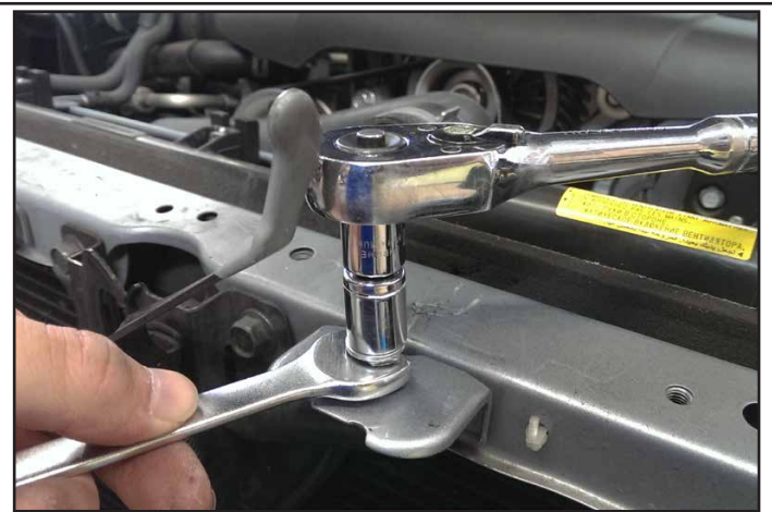
Attach (2) Rivnuts to each of the metal tabs on the upper radiator support. Use a 9/16" Wrench to hold the nut while tightening with a 7/16" Wrench or Socket.
