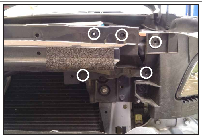
Remove the upper bumper beam by removing indicated bolts.
