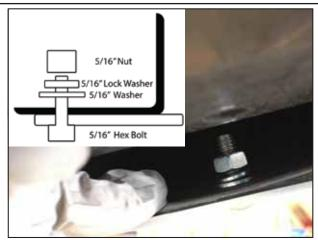
After aligning the splitter holes to the OEM bumper holes, fasten with (1) 5/16" Buttonhead Bolt, (1) Flat Washer, (1) Lock Washer, and (1) Hex Nut on each hole. The OEM plastic structure's holes will self-locate itself into the exposed bolt shaft.
