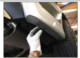
Remove (3) plastic rivets on each side, that hold the bumper to a plastic structure to allow easier access behind the bumper for installation.
