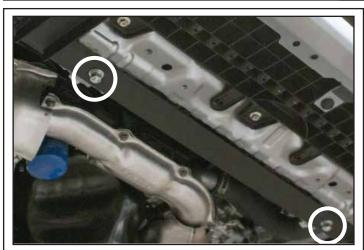
Attach the lower brace to the bolt plates using (1) 3/8" Flat Washer, (1) 3/8" Lock Washer, and (1) 3/8" Hex Nut on each side.
