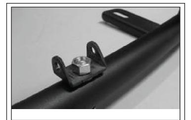
**Optional**: Attach (1) light bracket to the light bar using (1) 3/8"-16 x 1.75" Hex Bolt, (2) 3/8" Flat Washer, and (1) 3/8" Hex Nut per side. (**PIAA** light bracket shown)
