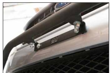
Attach the light bar to the upper bracket using (1) 3/8" x 1" Hex Bolt, (2) 3/8" Flat Washers, and (1) 3/8" Hex Nut on each side.
