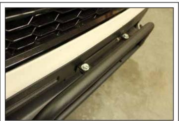
Check fitment, tighten all hardware, and re-attach splash guard. See below for cutting instructions.
