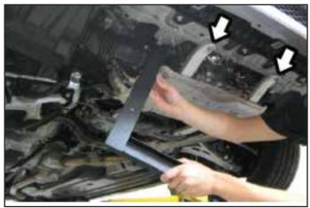
**WRX:** Slide the lower brace on by inserting it from the passenger side, then rotating it to clear the frame, engine, and turbo. **Tip:** You may want to lower the chassis brace shown above to ease install of the lower brace. Be sure to reinstall it once the lower brace is installed.
