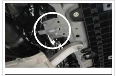
Remove the splash guard and locate the two indicated slots on the frame. Insert (1) 3/8" Bolt Plate in each slot. **WRX Shown**
