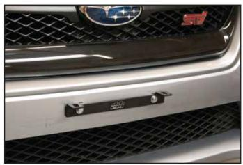
Attach the License Bracket to the bumper via the license plate holes using (2) 1/4" Lag Screws and (2) 1/4" Flat Washers.
