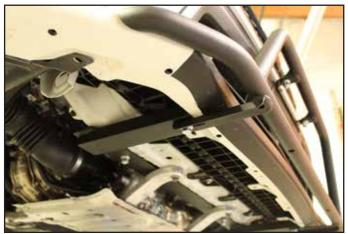
Attach the light bar to the lower brace using (1) 3/8" x 1" Hex Bolt, (1) Lock Washer, and (1) Flat Washer on each side.
