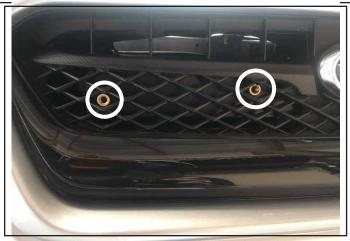
Press the Backing Plate into the grill. Check that the Rivnuts are inserted into the hexes shown.
