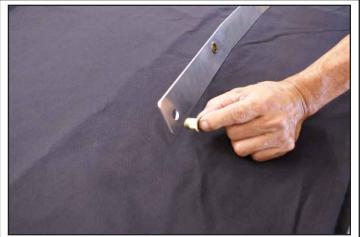
Insert (4) 5/16" Rivnuts through each hole in the Backing Plate. Ensure that the Rivnut heads are on the face that bends towards you.
