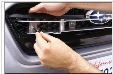
Fasten the Light Plate with (4) 5/16" Buttonhead Screws and Flat Washers. Reach through the grill to hold the Rivnuts in place.
