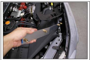
Insert Backing Plate with the Rivnuts protruding forward through the Plate. Note that the center rivnuts sit higher than the outer rivnuts.
