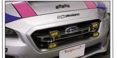
Attach, wire, and test Driving Lights before re-attaching the plastic bumper piece. (Baja Designs S2 LED lights shown.)
