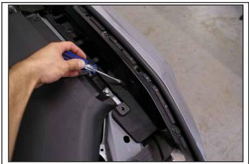
Remove the clips holding the plastic upper bumper piece and pry away the passenger side.
