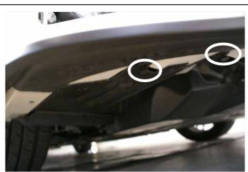
Remove (2) Pop-clips under each side splash shield. This allows you to reach behind the fog light to remove/install the screws.
