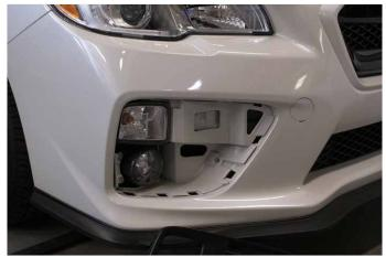
The tabs are placed around the outer perimeter of the fog bezel. It is recommended to pull from the middle rib of the fog cover.
