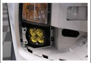
Install the Fog Light into the bumper. Install the inner tabs first, then attach the 1/4" hardware.
