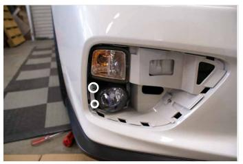
Remove the OEM Fog assembly with a screw driver. The two screws are positioned on the outer edge of the fog light.
