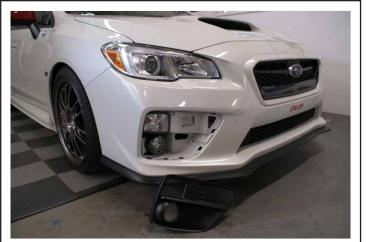
For vehicles **without** foglights installed, cut the bezel to create a circular hole for the fog lights to shine through. Alternatively, source OEM fog covers with the opening.
