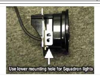
Attach new foglight to Light Conversion Bracket like shown above. Repeat on passenger side.
