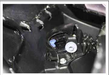
Unplug the foglight harness and undo the plastic screw and (2) M6 bolts shown above (keep for later).
