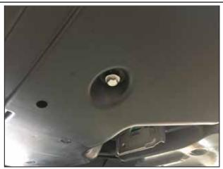
Reinstall splash guard with included M8 x25mm bolts and factory plastic clips. Tighten M8 bolts to 23 ft-lbs.
