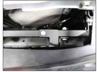
Use 1/4-20x1.25" hex bolt and 1/4-20 Nylock Nut to assemble Upper Bracket to the Upper Brace.
