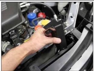
Attach Upper Support Brackets to Upper Brace as shown. Note orientation of the bracket.
