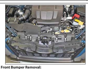
Remove the fasteners and unplug the harness at the air diverter panel above the front bumper.
