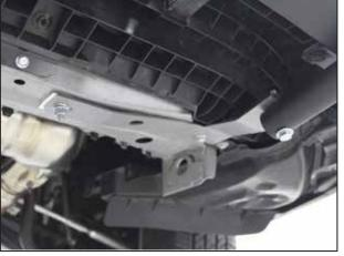
Attach Light Bar to Lower Brackets with (1) 3/8"-16 x2.5" Hex Bolt, (2) 3/8" Washers, (1) 3/8" Lock Washer, and (1) 3/8" nut, per side. Tighten all bolts. Torque 3/8" hardware to 33 ft-lbs, 5/16" to 19 ft-lbs, and M6 to 11 ft-lbs. (Wilderness models, see Addendum A Step 11-12, prior to doing this step)
