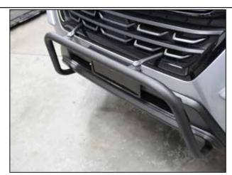
Attach Light Bar to Upper Tube Supports with (1) 3/8"-16 x1" Hex Bolt, (2) 3/8" Washers, (1) 3/8" Lock Washer, and (1) 3/8" nut, per side. Tighten all bolts. Torque 3/8" hardware to 33 ft-lbs, 5/16" to 19 ft-lbs, and M6 to 11 ft-lbs. (Wilderness models, see Addendum A - Step 11-12, prior to doing this step)
