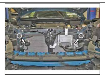
Front bumper cover removed. Remove M6 screws shown (same screws shown in Step 7 of the original instructions).
