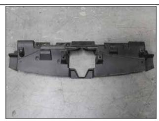
Remove upper radiator shroud to gain access to mounting points for the Upper Brace and installation.
