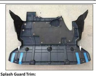
Trim splash guard material **inside** the marked area. *Pictured: Inner Side* Note: Cut 1" from the rib (shown above).
