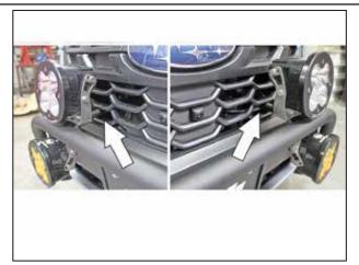
Reinstall front bumper with the upper bracket entering through the lower holes in the grille.
