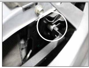
Attach Upper brace to the same holes in Step 7 using (1) 1-1/4" Aluminum Spacers and (1) M6x50mm Bolt, per side.
