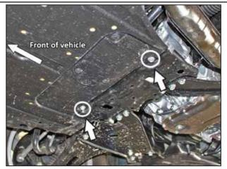
**Splash Guard Removal Cont'd:** Remove the screws toward the rear of the splash guard.
