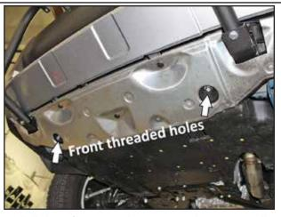
Reinstall all plastic fasteners in their respective locations. Install (1) M8 Flange Bolt and (1) 5/16" (Wide) Flat Washer to each of the threaded holes near the front of the splash guard. Reuse the factory screws in the rear screw locations.
