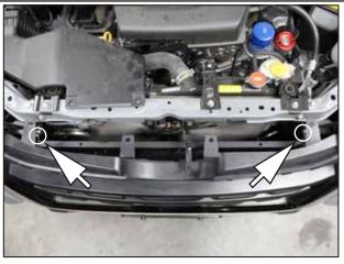
Remove the (2) M6 bolts shown above (L+R). These holes are where the Upper Brace will attach to.
