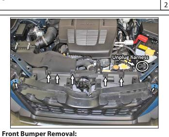
Remove the fasteners and unplug the harness at the air diverter panel above the front bumper.
