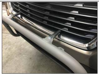
Attach Light Bar to Upper Brace with (1) 3/8"-16 x 1.00" Hex Bolt, (2) 3/8" Flat Washers, (1) 3/8" Lock Washer, and (1) 3/8" Hex Nut per side. Assemble loosely.
