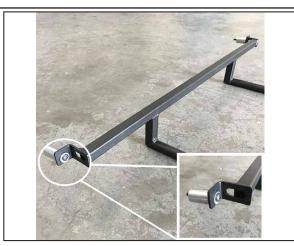
Attach Upper brace to the same holes in Step 7 using (1) 1-1/4" Aluminum Spacers and (1) M6x50mm Bolt, per side.
