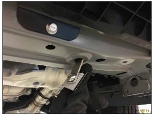
Insert (2) 5/16" Bolt Plates through the holes shown in Step 1.
