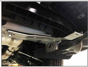
Install Lower Brackets (L+R) using the factory M6 bolt (do not tighten all the way). Install (1) 5/16" Flat Washer, Lock Washer, and Hex Nut onto the 5/16" Bolt Plate.
