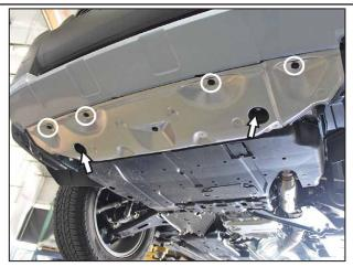
**Splash Guard Removal:** Remove the fasteners and screws which hold the splash guard in place.
