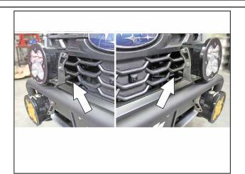
Reinstall front bumper with the upper bracket entering through the lower holes in the grille.
