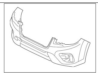
Remove front bumper cover to gain access to mounting points for the Upper Brace.
