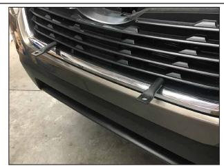
Reinstall air diverter and front bumper cover.
