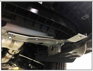
Install Lower Brackets (L+R) using the factory M6 bolt (do not tighten all the way). Install (1) 5/16" Flat Washer, Lock Washer, and Hex Nut onto the 5/16" Bolt Plate. Repeat on the passenger side.
