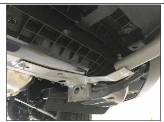
Attach Light Bar to Lower Brackets with (1) 3/8"-16 x2.5" Hex Bolt, (2) 3/8" Washers, (1) 3/8" Lock Washer, and (1) 3/8" nut, per side. Tighten all bolts. Torque 3/8" hardware to 33 ft-lbs, 5/16" to 19 ft-lbs, and M6 to 11 ft-lbs.
