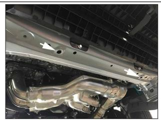
Remove the front splash guard and locate the holes shown above.
