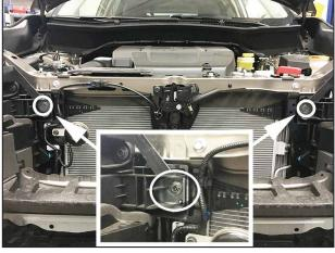
Remove the (2) M6 bolts shown above (L+R). These holes are where the Upper Brace will attach to.
