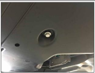
Reinstall splash guard with included M8 x25mm bolts and factory plastic clips. Tighten M8 bolts to 23 ft-lbs.
