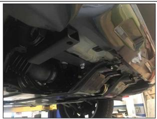
Insert Lower Mounting Brace with the C-channels pointed up; slide up and over the car's frame. Enter through the passenger side. Attach to Bolt Plates with (1) 3/8" Flat Washer, (1) Lock Washer, and (1) Hex Nut per side.
