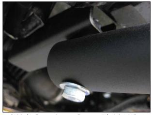
Attach Light Bar to Lower Brace with (1) 3/8" x 2.50" Hex Bolt, (2) Flat Washers, (1) Lock Washer, and (1) Hex Nut per side.
