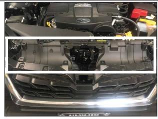
Open the hood and remove the air deflector. Loosen the front bumper cover to access the headlight mounts.
