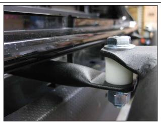
Attach Light Bar to Upper Brace with (1) 3/8" x 1.75" Hex Bolt, (1) Nylon Spacer, (2) Flat Washers, (1) Lock Washer, and (1) Hex Nut per side.
