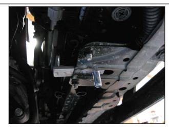
Insert (2) 3/8" Bolt Plates through the slots shown.
