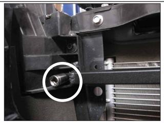
Remove the lower bolt attached to the headlight housing shown. Attach Upper Mounting Brace with the same bolt.
