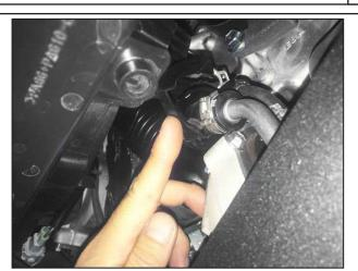
Remove the plastic clip covering the hose in front of the engine. Reattach after inserting Lower Mounting Brace.
