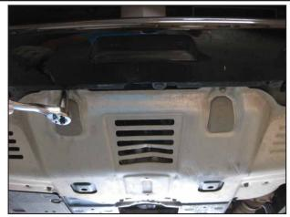
Remove the front splash guard. XT splash guard shown.
