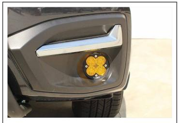
Reinstall splash guard, and front bumper cover (if removed) using factory plastic clips. *Pictured: Completed Assembly.*
