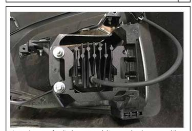
Attach new foglight assemblies to the bumper like shown above using the included 1/4"-20 hardware.
