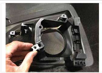
Remove the factory foglight and the metal j-clip shown above. Repeat on the passenger side.
