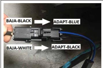
**Assembling Wire Adapter (Optional):** Note that the provided dual-application adapter requires to reverse the color polarity on this car. Test polarity before assembling wires to the Baja Designs connector. Note that the adapter connects to OEM connecter easier on one orientation than the other.
