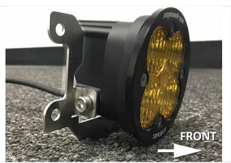
Attach the new foglight in the Light Conversion Bracket like shown above. Repeat on the passenger side.
