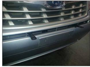
Insert the Upper Brace behind the bumper cover. Slide the tabs through the openings under the grill.
