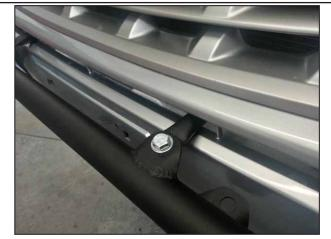
Attach the Light Bar to the Upper Brace with (1) 3/8" x 1" Hex Bolt, (2) Flat Washers, (1) Lock Washer, and (1) Hex Nut per side.
