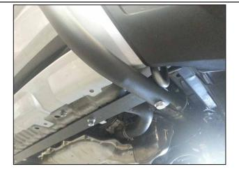
Attach the Light Bar to the Lower Brace with (1) 3/8" x 2.5" Hex Bolt, (2) Flat Washers, (1) Lock Washer, and (1) Hex Nut per side.
