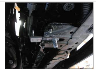
Remove the lower splash guard and insert (2) Bolt Plates into the slots shown.
