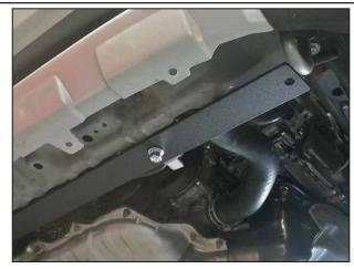
Attach the Lower Brace with (1) 3/8" Flat Washer, (1) Lock Washer, and (1) Hex Nut per side.
