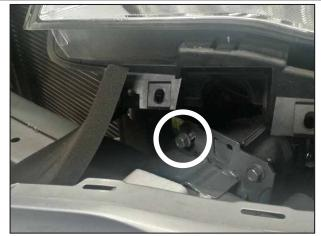
Partially remove the front bumper from the top and remove the (2) bolts on the bumper beam shown above.
