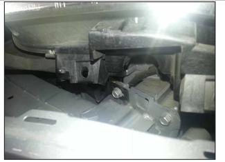
Attach the Upper Brace to the bumper beam with the factory bolts from Step 3.
