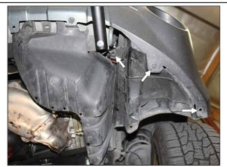
Remove the fog light splash guard by unfastening the plastic clips holding it in place using a panel removal tool.
