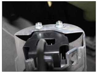
Fasten the carriage bolts with (1) Flat Washer and (1) Kep Nut on the threaded end of each bolt.
