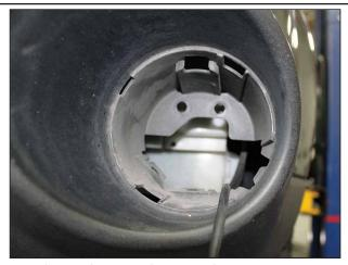
Remove factory fog light, if present. If vehicle did not come with fog lights, remove cap on bumper to access fog light hole. To do this, pry carefully with panel removal tool while pushing from behind with your other hand.
