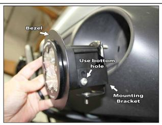
Assemble new fog light into mounting bracket. First, slip on the fog light bezel onto fog light housing, then attach fog light to the mounting bracket via included screws. Fasten screws using 5/32" hex key.
