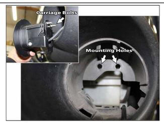
Insert the fog light assembly into the fog light hole in the front bumper. Align the top two carriage bolts with the holes in the bumper.
