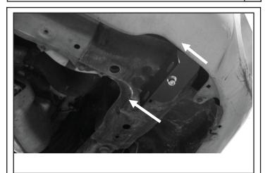
Attach the mounting brackets with 3/8" Flat Washer, Lock Washer, and Hex Nut. Orient the bracket such that the bent tab is inboard of the car.
