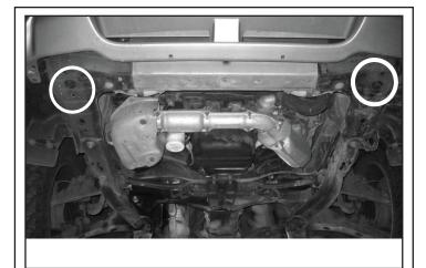
Remove splash guard and locate the indicated holes.
