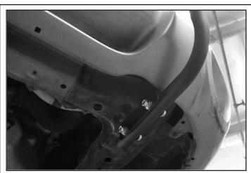
Attach the light bar to the brackets with (2) 3/8"x16 -2" Hex Bolts, (4) Washers, (2) Lock Washer, and (2) Hex Nut on each side. Loosely fasten to allow adjustments
