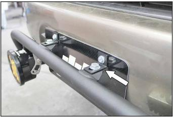
**06-08 Forester:** Attach license plate L-brackets in the orientation shown. The brackets sit on top of the light bar. Torque nuts to 32 ft-lbs.
