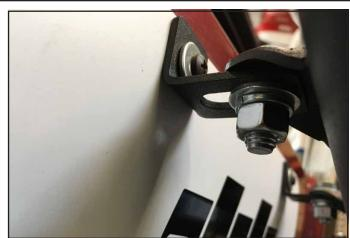
Torque 3/8" hardware used on the top and bottom mounting locations of the light bar assembly to 32 ft-lbs.
