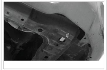
Locate the large hole on the frame and insert 3/8" Bolt Plate with the threaded shaft protruding through the smaller hole.
