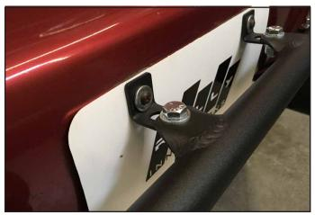
Attach license plate L-brackets on the front bumper using (2) screws, (2) 1/4" washers, and (2) 3/8"-16 x 1" bolts, (4) 3/8" washers, (2) 3/8" lock washers, and (2) 3/8-16 nuts
