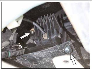
Light assembly installed in the bumper using (1) 1/4"-20 x 3/4" Hex Bolt, (1) 1/4" Split Lock Washer and (1) 1/4" SAE Flat Washer into each mounting point (shown by arrows).
