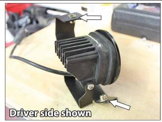
The mounting points onto the bumper are shown above. (Driver side shown).
