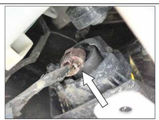
Remove factory fog light by first unplugging the connector.
