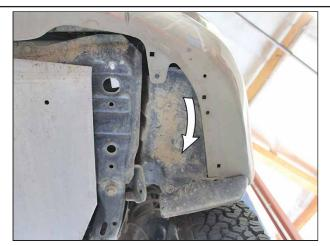
Remove fasteners securing fog light splash guard and pull guard down and back to gain access to the area behind the fog light.
