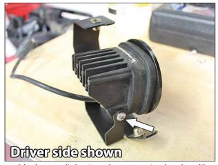
Assemble the new lights into the conversion brackets like shown. Arrow indicates mounting points for lights.
