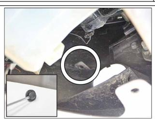
On top of the light there is a plastic fastener that attaches the light to the bumper tab shown. To remove this, use a small flat head screwdriver to release the rivet. This step has some slight difficulty but is still possible to do without complete removal of front bumper.
