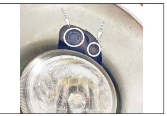
The fastener on the left can be removed using a panel removal tool (remove the center pin first). Remove the bolt on the right using a 10mm socket wrench.
