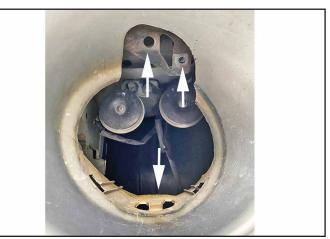
Remove factory fog light, by unplugging the fog light from the main harness and removing (3) fasteners located in the areas shown above.
