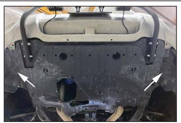
Remove splash guard to gain access to the fog light area behind the front bumper.
