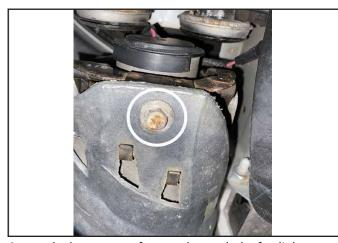
Access the lower screw from underneath the fog light.
