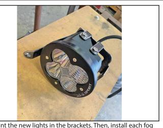
Mount the new lights in the brackets. Then, install each fog light assembly onto the car.
