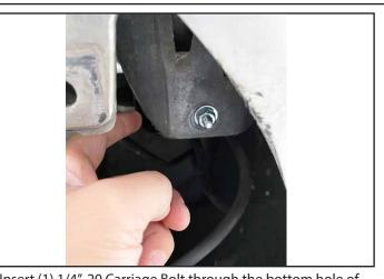
Insert (1) 1/4"-20 Carriage Bolt through the bottom hole of the bracket so that the threads are pointing down towards the ground. Fasten with (1) 1/4" Flat Washer and (1) 1/4" Kep Nut.
