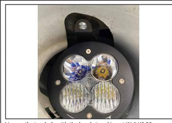
Line up the top hole with the bracket and insert (1) 1/4"-20 Carriage Bolt through the face of the bracket. Carefully reach behind the hole (from underneath and behind the fog light) to fasten with (1) 1/4" Flat Washer and (1) 1/4" Kep Nut.
