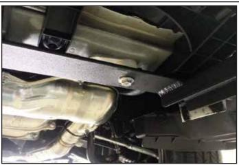
Install the mounting brace, using the (1) round spacer, (1) M8 bolt, (1) 5/16 lock washer, and (1) 5/16 washer, per side. Tighten to 15 lb-ft.
