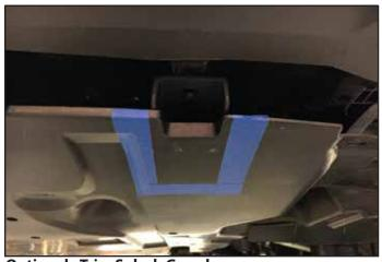
Optional - Trim Splash GuardLoosely attach the splash guard. Mark area around the<br/>mounting brace to trim for clearance. Mounting brace<br/>shown and light bar unmounted for clarity.7
