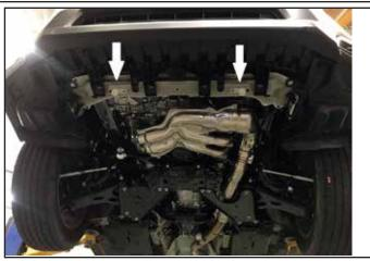
Remove the splash guard. Identify the two mounting points (indicated by arrows) to install the mounting brace. Remove the OEM plastic spacer - use the round spacer provided in its place.
