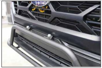
Attach the lightbar from the top using the license plate bracket, with (2) 3/8" washers, (1) 3/8" lock washer, (1) 3/8-16 x1.5" bolt, and (1) 3/8-16 nut, per side. Keep loose for adjustments.
