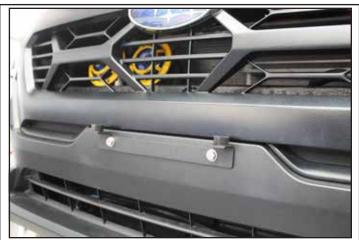
Install the license plate mounting bracket, using the supplied 1/4" lag screws and 1/4" washers. Place nylon spacers on top of bracket as shown.
