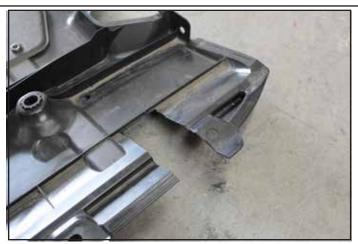
The trimming area is up to the 2nd plastic rib (as shown above). The approximate area is 5 inches by 2.5 inches, for each side of the splash guard.
