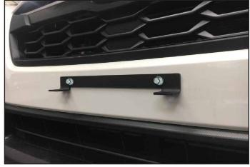
Install the license plate mounting bracket, using the supplied 1/4" lag screws and 1/4" washers.
