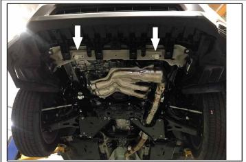
Remove the splash guard. Identify the two mounting points (indicated by arrows) to install the mounting brace. Remove the OEM plastic spacer - use the round spacer provided in its place.
