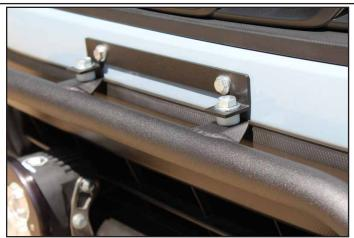
Attach the lightbar from the top using the license plate bracket, with (2) 3/8" washers, (1) 3/8" lock washer, (1) 3/8"-16 x1.5" bolt, (1) nylon spacer and (1) 3/8"-16 nut, per side. Keep loose for adjustments.
