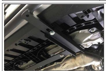
Attach the lightbar from the bottom, using (1) 3/8" washer, (1) 3/8" lock washer, and (1) 3/8-16 x3/4" bolt, per side. Keep loose for adjustments.
