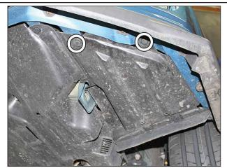
Pull down the fog light splash guard by removing the fasteners shown above with a Panel Removal tool.
