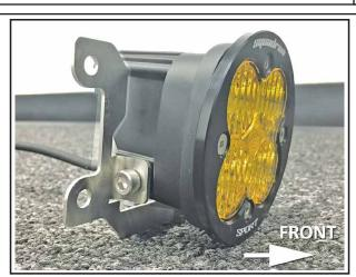
Assemble the new lights into the conversion brackets like shown.
