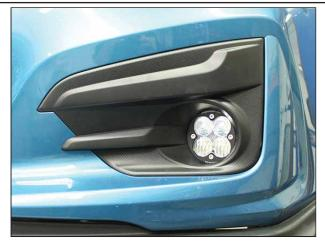
Review the light position in the front bumper. Reinstall the fog light bezel on the bumper.
