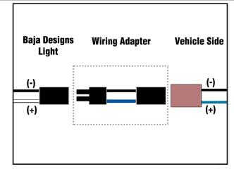
**Installing Pigtail Adapter (Optional):** Note the orientation of the optional pigtail adapter.
