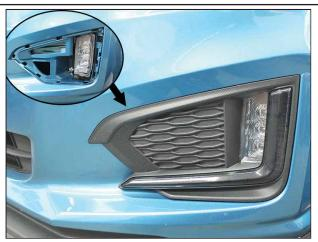
Remove the factory fog light bezel by prying carefully around it with a plastic panel removal tool.
