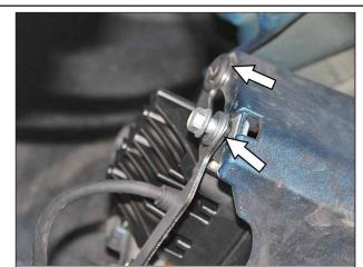
Install the new light assemblies in the reverse order of the factory light removal. Insert the factory 10mm-head screw in its original position with the (2) 1/4" Flat Washers on it. Reinstall the factory plastic fastener in its original position.
