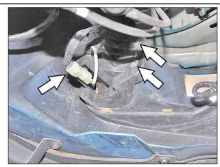
Remove the factory fog light by undoing the factory fasteners and unplugging it from the wire harness. One of the fasteners is a 10mm-head screw and the other is a plastic screw to be undone with a stubby flat head screwdriver.
