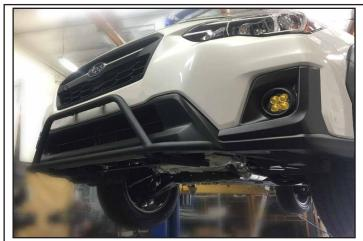
Confirm alignment throughout the lightbar assembly. Tighten 3/8-16 hardware to 30 ft-lb.
