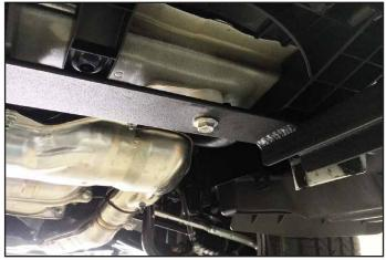
Install the mounting brace, using the (1) round spacer, (1) M8 bolt, (1) 5/16 lock washer, and (1) 5/16 washer, per side. Tighten to 15 lb-ft.
