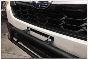
Attach the lightbar from the top using the license plate bracket, with (2) 3/8" washers, (1) 3/8" lock washer, (1) 3/8-16 x1" bolt, and (1) 3/8-16 nut, per side. Keep loose for adjustments.
