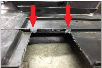
For each opening, trim 2 notches approximately 3/8 to 1/2 inch wide. This is to clear the edges of the mounting brace. Clean up edges, and reinstall the splash guard. Note: The mounting brace uses 2 points of the splash guard already.
