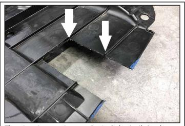
The trimming area is up to the 2nd plastic rib (as shown above). The approximate area is 4 inches by 2.5 inches, for each side of the splash guard.
