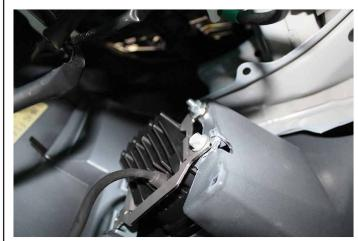
Fasten locking nut onto top bolt and insert factory M6 flange-head bolt into bottom right hole and fasten down. Tighten hardware.
