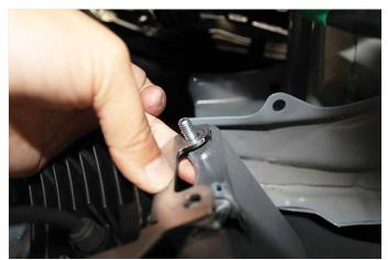
Insert the new foglight assembly into the front bumper in the reverse order of removal of the factory foglight. Slide the left tabs into the mounting slots and slide the top right hole onto the 1/4" bolt. Tip: Support the back of the top bolt with your finger as you fasten the locking nut onto the assembly.
