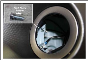
Insert the 1/4" hex bolt and internal lock washer into the top mounting hole in the bumper, as shown above.
