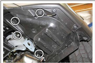
Remove splash guard underneath foglight on driver and passenger sides to gain access to foglight area. (Save factory hardware and clips for later).
