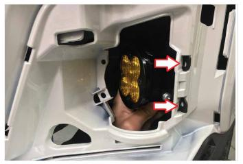
Slide in the Baja Designs light and Rally Innovations bracket assembly into the (2) slots, shown above.
