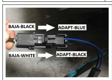
Assembling Wire Adapter: Note that the provided dual-application adapter requires to reverse the color polarity on this car. Simply switch wire when assembling wires to the Baja Designs connector. Note that the adapter connects to OEM connecter easier on one orientation than the other.
