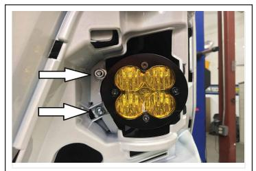
Top arrow - install using (1) 1/4-20 bolt, (2) 1/4 washers, (1) lock washer, and (1) 1/4-20 nut.
