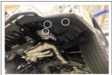
Remove (2) plastic rivets and (1) screw, to allow access behind the fog light.
