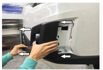
Remove the fog light bezel, by pulling firmly and directly forward.
