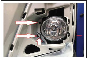
Remove OEM hardware. Top long arrow - use a short screwdriver to remove plastic rivet. Bottom long arrow - use socket to remove bolt. Bottom short arrow - remove clip-on nut.
