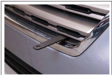
Carefully reattach the bumper cover with the Upper Brackets through the grill as shown.
