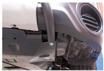
Cut the splash guard by following the outer crease until the bar clears.
