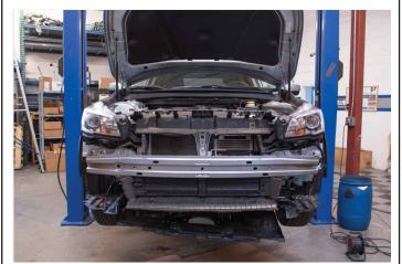
Remove the front bumper cover and the foam piece in front of the bumper beam.
