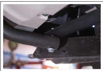
Attach the Light Bar to the Lower Brace with (1) 3/8" x 2.5" Hex Bolt, (2) Flat Washers, (1) Lock Washer, and (1) Hex Nut.
