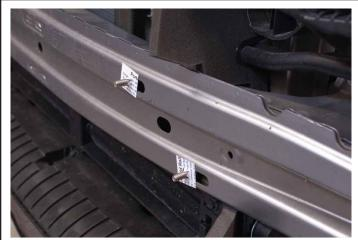
Insert (4) 5/16" Bolt Plates into the holes shown. Slide the Bolt Plates towards the center of the vehicle.
