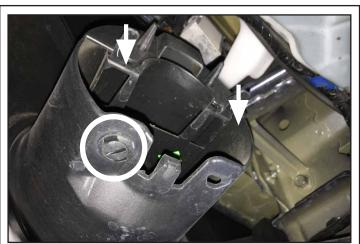
Carefully remove (1) plastic rivet from the fog light cover. Pull down (2) plastic tabs to release the fog light cover. For vehicles with OEM fog lights installed: remove the hardware securing the fog light assembly (2 nuts and 2 plastic rivets), including the connecting plug.
