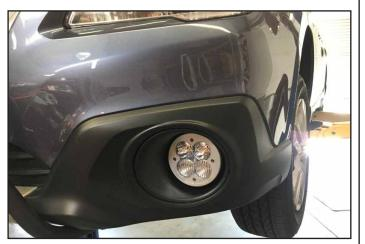
Double-check installation and re-attach the splash guard with the plastic rivets.
