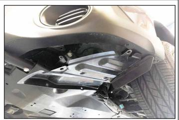
Carefully pull down plastic splash guard to access the fog light hardware.
