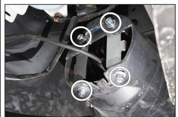
Install (1) 1/4"-20 x 5/8" carriage bolt, (1) washer, (1) lock washer, and (1) hex nut on (2) bottom mounting points. Install (1) washer, (1) lock washer, and (1) 1/4"-20 hex nut on (2) top mounting points.
