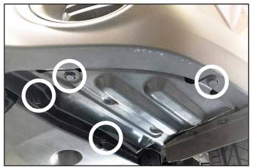
Carefully release (4) plastic rivets from the splash guard to access the fog light area.
