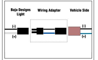
**Diagram - Wiring Adapter (Optional):** Sometimes the Wiring Adapter wire color will not match the ground wire color (-) from the vehicle, this is fine as long as the ground mates to the
