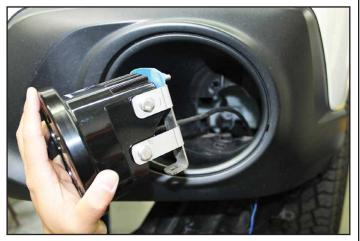
Place the upgraded fog assembly into the fog light pocket until the bracket meets the plastic face of the bumper cavity.
