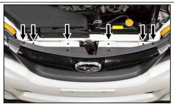
Remove bumper and grille clips. Remove splashguard underneath the engine bay.
