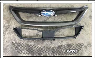
The grille consists of three pieces. Top to bottom: Grille frame, mesh retainer, and mesh.
