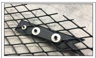
If retaining the mesh grille, you will need to reposition the "WRX" emblem. Carefully remove emblem lock washers with a small flathead screwdriver and pliers. Reposition emblem to your liking, then reinstall mesh into the grille frame in the reverse order of step 10.
