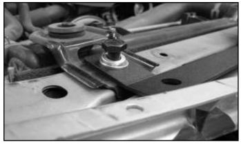
Bolt the bent tab of the grille bracket to the radiator mounting bracket using a 12mm socket and (1) M8x25mm Flanged Head Bolt. Repeat on other bracket.
