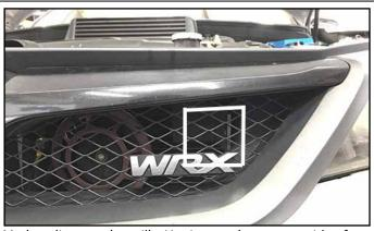
Mark cutlines on the grille. Use image above as a guide of what to cut to make space for the bar to slide through the grille for mounting to the Upper Mounting Bracket. Emblem will need to be repositioned.
