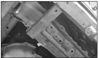
Attach the Lower Mounting Brace to the bolt plates using (1) 3/8" Flat Washer, (1) 3/8" Lock Washer, and (1) 3/8" Hex Nut, per side. Use a 9/16" socket/wrench to fasten hardware.
