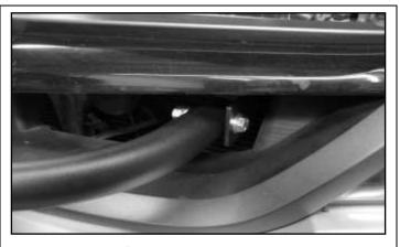
Attach each side of the light bar to the Upper Mounting Bracket behind the grille with a 9/16" socket using (1) 3/8"-16 x2" Hex Bolt, (2) 3/8" Flat Washer, (1) 3/8" Lock Washer, and (1) 3/8" Hex Nut. Repeat on the other side.
