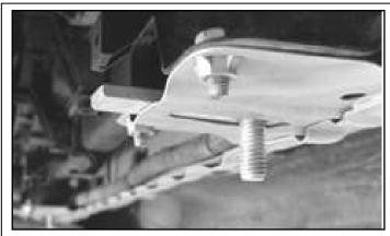
Beneath the vehicle, locate the two slots on the chassis beneath the radiator on the driver and passenger side and insert (1) 3/8" Bolt Plate into each slot with the threaded shaft facing down.
