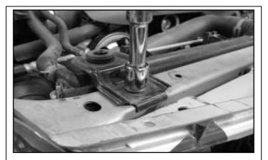
Remove the factory bolts for the radiator mounting brackets (R+L side) using a 12mm socket.
