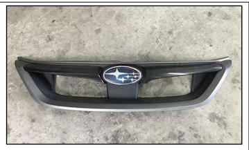
If discarding entire mesh piece, reinstall the mesh retainer into the grille frame using the same screws removed in step 9.
