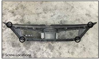
Remove the grille from the bumper cover by removing the screws behind the grille in the areas shown above. Note: Screw location may vary depending on the year of your vehicle.
