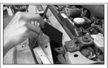
Install the Upper Mounting Bracket, as shown, by carefully pulling the bumper cover away from the car (if you have not removed it) and inserting the bracket behind it. The small bent tab should sit over the radiator mounting bracket, and the forward leg fits in the space of the grille.
