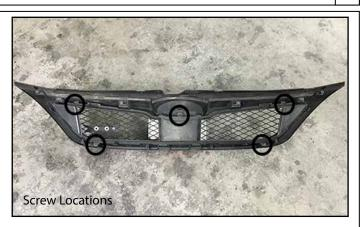
To remove the mesh from the grille, remove the screws outlined above. Note: Screw locations may vary depending on the year of your vehicle.
