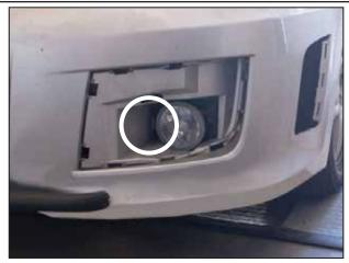
Remove the (2) Phillips screws on the inner side of the fog light.
