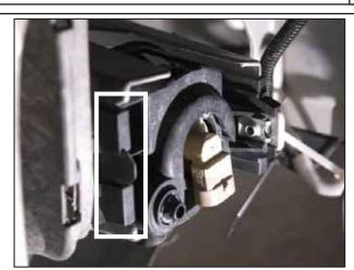
Push in the (2) tabs near the location identified above and carefully pull the fog light backwards.
