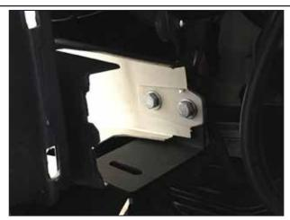
Attach the Mounting Bracket with (2) 5/16" Hex Bolts, (4) Flat Washers, (2) Lock Washers, and (2) Hex Nuts. Note that the slotted flange is on the bottom side.
