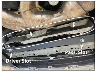
Non-turbo models: Remove heatshield using a 10mm socket wrench to unfasten the (2) screws indicated by the arrows. Insert (1) 3/8" Bolt Plate into driver side slot and (1) 3/8"-16 x 1" Hex Bolt with a (1) 3/8" USS Flat Washer (large size Flat Washer) into the passenger side slot.
