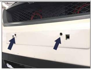
Locate (2) license plate holes on the front bumper, as shown above.
