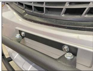
**All other models:** Attach Light Bar to License Plate Bracket with License Plate Bracket flanges under the bar flanges.
