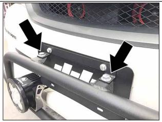
**08-10 STI:** Attach Light Bar to License Plate Bracket with (1) 3/8"-16x1" Hex Bolt, (2) 3/8" Flat Washers, (1) 3/8" Lock Washer, and (1) 3/8" Hex Nut, per side. **Note:** License Plate Bracket flanges are on top of the bar flanges.
