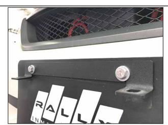
Attach License Plate and License Plate Bracket to the front bumper cover with (1) 1/4" Lag Screw and (1) 1/4" Flat Washer, per hole.
