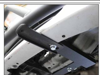
Attach Light Bar with (1) 3/8"-16x1" Hex Bolt, (1) 3/8" Lock Washer, and (1) 3/8" Flat Washer per side.
