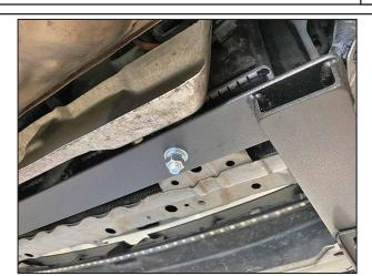
Attach Lower Brace with (1) 3/8" Flat Washer, Lock Washer, and Hex Nut per side. Do not tighten yet - allow the brace to move freely from front-back along the slots.
