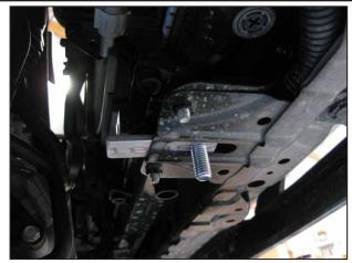
Remove the plastic Splash Guard. **Turbo models:** Insert (2) 3/8" Bolt Plates into the slots shown.
