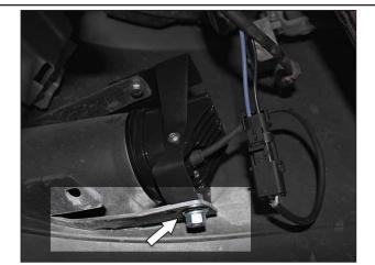
Enlarge the hole on the plastic bumper mounting tab with a 3/8" drill bit to accomodate the new 3/8" mounting hardware.
