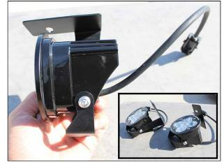
Take the new mounting brackets and assemble the fog lights in them (as shown above) with the included fog light hardware.
