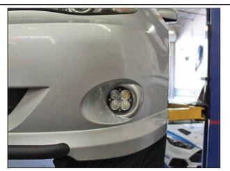
Confirm the position of the light in the bumper fog light hole is center and tighten all hardware. Repeat the process on the passenger side.
