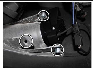
Remove the factory fog light by unfastening the factory hardware. There are (3) fasteners that need to be removed to free the fog light. Note: Aftermarket Fog Light shown, factory fog light will look different but attaches to the same mounting points.
