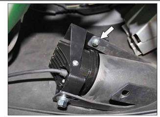
Insert (1) 1/4"-20 x 3/4" Hex Bolt through the top bumper mounting tab and fog light bracket. Fasten on the other end with (1) 1/4" Flat Washer, Split Lock Washer, and Hex Nut.
