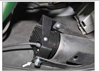
The driver side assembly mounts as shown. Insert (1) 3/8"-16 x 1" Hex Bolt and (1) 3/8" Flat Washer through the fog light bracket and bumper mounting tab. Then fasten with 3/8" Flat Washer, Split Lock Washer and Hex Nut.
