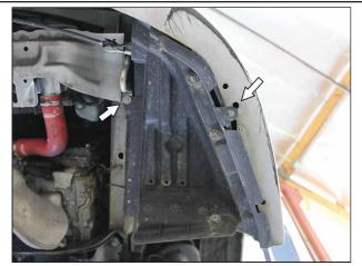
Remove fog light splash guard by unfastening the plastic clip and 10mm head screw securing it and pulling it downward.
