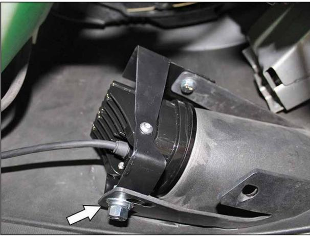
The driver side assembly mounts as shown. Insert (1) 3/8"-16 x 1" Hex Bolt and (1) 3/8" Flat Washer through the fog light bracket and bumper mounting tab. Then fasten with 3/8" Flat Washer, Split Lock Washer and Hex Nut.
