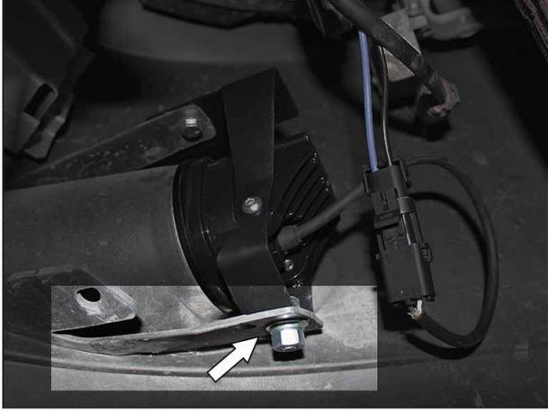
Enlarge the hole on the plastic bumper mounting tab with a 3/8" drill bit to accommodate the new 3/8" mounting hardware.
