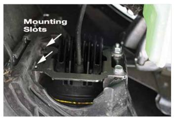
Note: There are two open slots in the bumper that the light bracket mounting tabs (left) slide into.
