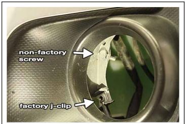
Remove the factory foglight and retain factory fasteners for reuse on new light assembly. Repeat on the passenger side. (If factory hardware is not present, use included 1/4" hardware as necessary; our test vehicle still had the factory j-clip but was missing the upper mounting fastener)
