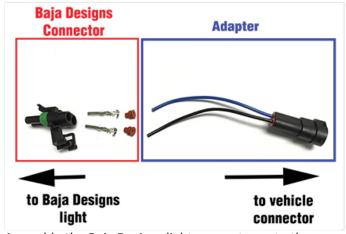
Assemble the Baja Designs light connector onto the optional pigtail adapter in the order shown above.
