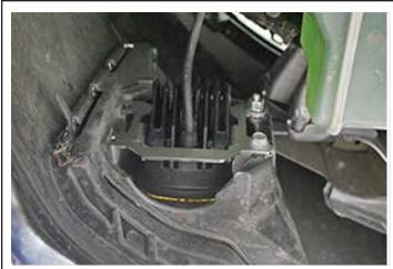
Attach new foglight assemblies to the bumper like shown above using the included 1/4"-20 hardware (if factory hardware is not available).
