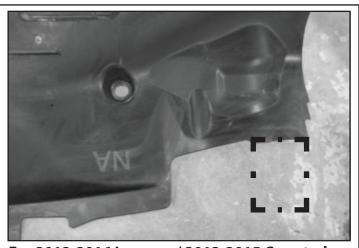
For 2012-2016 Impreza / 2013-2015 Crosstrek: Cut the splash guard as shown above and reattach.
