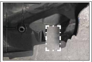
For 2012-2016 Impreza / 2016-2017 Crosstrek: Cut the splash guard as shown above and reattach.
