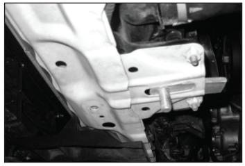
Remove the splash guard and insert (2) 3/8" Bolt Plates into the (2) slots shown above.
