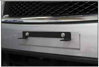
Attach License Plate Bracket to existing holes in bumper cover using (1) 1/4" Lag Screws and (1) Flat Washer for each mounting hole.
