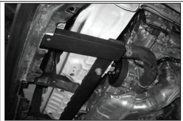
Attach the Mounting Brace to the Bolt Plates using (1) 3/8" Flat Washer, (1) Lock Washer, and (1) Hex Nut per side. Trim the bumper cover as shown.
