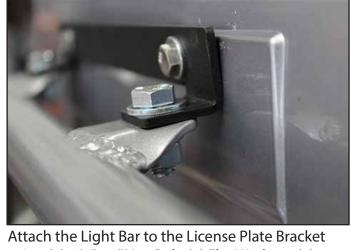
Attach the Light Bar to the License Plate Bracket using (1) 3/8" x 1" Hex Bolt, (2) Flat Washers, (1) Lock Washer, and (1) 3/8" Hex Nut per side. Keep loose for adjustments.
