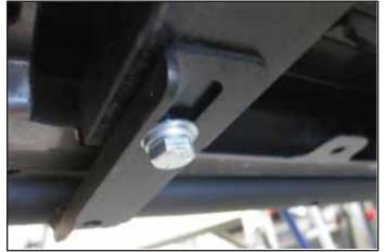
Attach Light Bar to Mounting Bracket using (1) 3/8" x 1" Hex Bolt, (1) Lock Washer, and (1) Flat Washer
