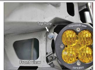
Install new light assembly using the same mounting points as the original. Fasten the top hole (shown above) with (1) 1/4"-20x 3/4" Hex Bolt, (2) 1/4" Flat Washer, (1) 1/4" Split Lock Washer, and (1) 1/4"-20 Hex Nut.
