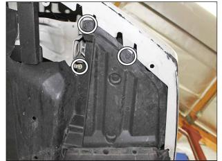
Remove factory fasteners securing the splash guard to gain access to the fog light area.
