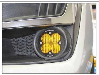
Reinstall the fog light bezel & splash guard and repeat steps on the opposite side fog light.
