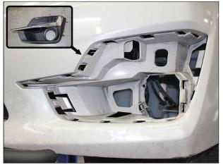
Remove fog bezel from the bumper. Use a Panel Removal Tool, if necessary, to gently pry on the bezel fingers behind the front bumper to displace it from its location.
