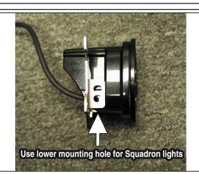
Assemble the light and light conversion bracket together.
