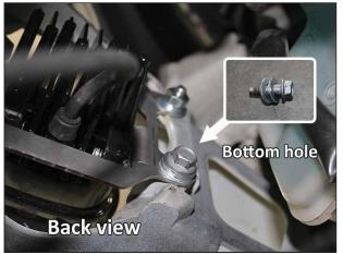
For the bottom hole, reinstall the factory 10mm head bolt with (2) 1/4" Flat Washers.
