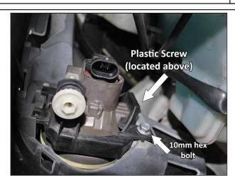
Remove the light by unfastening the 10mm head bolt and plastic screw shown above.
