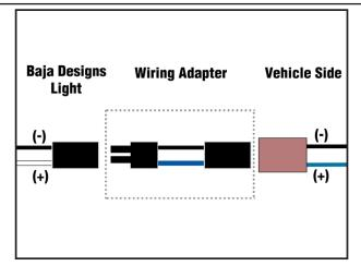
The wiring adapter installs between the vehicle harness and the light like shown above. The (-/+) on the light should coincide with the (-/+) on the vehicle harness and vice versa. Note: The -/+ on the light is black/white.
