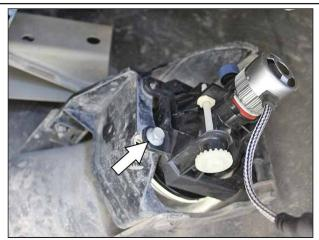
Unplug the factory fog light and remove the 10mm-thead screw fastening the light to the bumper (retain for use later).
