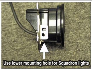
Assemble the fog light into the mounting bracket like shown.
