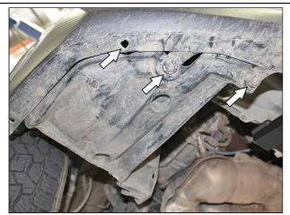
Remove the fog light splash guard to gain access to the fog light area by removing all fasteners with a panel removal tool.
