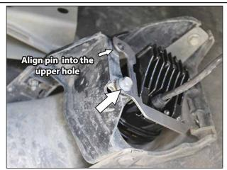
Install the new fog light assembly into the factory location in the reverse order of removal.
