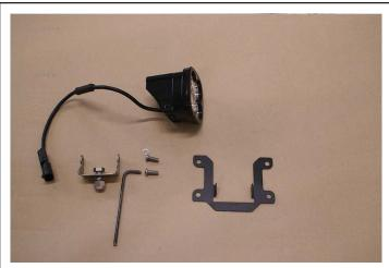
Remove the Baja Designs bracket and replace with Rally Innovations Light Conversion Bracket.
