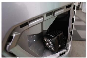
Slide the light conversion from the inner-side of the bumper cover.
