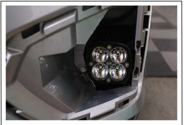
Attach the hardware to the bottom corner of the bumper cover to the bracket.
