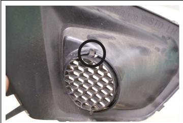
For Fog cover **without** foglights installed, remove the small cover. Press the circled tab down and push from the rear of the fog cover.
