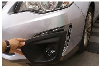
Carefully pull forward to release the tabs and pull the fog cover towards the front of the vehicle.
