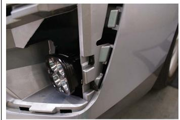
Then slide the outer tabs into the slotted hole on the bumper cover.
