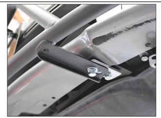
Attach the light bar to the spacer using (1) 3/8"-16x 1/2", (1) 3/8" Lock Washer, and (1) 3/8" Flat Washer. Tighten all 3/8" hardware to 33 ft-lbs.
