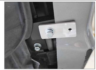
Attach the spacer to the lower brace using (1) 3/8"-16x 1.5" hex bolt, (1) 3/8" lock washer, and (1) 3/8" flat washer. Keep loose for now.
