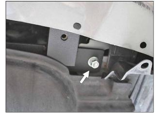
Attach the mounting brace to the lower bumper beam by using (1) 3/8 washer, (1) 3/8 lock washer, (1) 3/8 nut.
