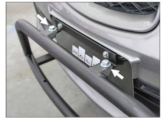
Attach the light bar to License Plate Bracket using (1) 3/8"-16x 1" hex bolt, (2) flat washer, (1) lock washer, and (1) 3/8" nut for each side.
