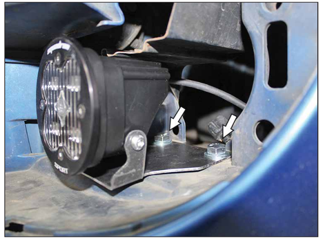
Insert (1) 5/16"-18 x 1" Hex Bolt and (1) 5/16" Flat Washer into each slot on the mounting bracket and fasten to the vehicle using (1) 5/16" Flat Washer, (1) 5/16" Lock Washer and (1) 5/16"-18 Hex Nut on the bottom side. (04-05 WRX shown)
