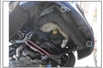
Remove factory splash guard. Locate holes on lower bumper beam.
