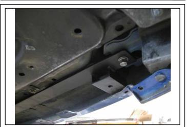
Attach the mounting brace to the lower bumper beam with (2) 3/8" Washers, (2) 3/8" Lock Washers, and (2) 3/8" Hex Nuts.
