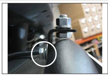
Attach L-Brackets to Skid Guard tube with (1) 5/16" Hex Bolt, (1) 5/16" Lock Washer, and (1) 5/16" Flat Washer through the slot of each bracket.
