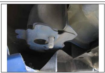
Locate the two holes in the lower bumper beam and insert (1) 3/8" Bolt Plate through each hole.
