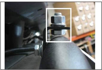
Assemble (2) L-Brackets with (1) 3/8"-.75" Hex Bolt, (1) 3/8" Lock Washer, and (1) 3/8" Hex Nut through the hole on each bracket.
