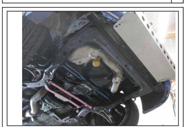
Attach Skid Guard to brace using (2) 3/8"-1" Hex Bolts, (2) 3/8" Lock Washers, and (2) 3/8" SAE Washers.
