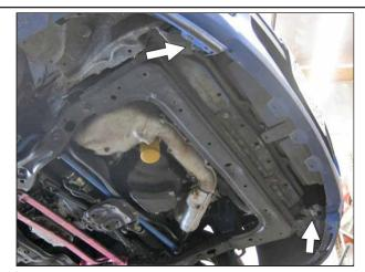
Remove the factory splash guard. Locate holes on lower bumper beam.
