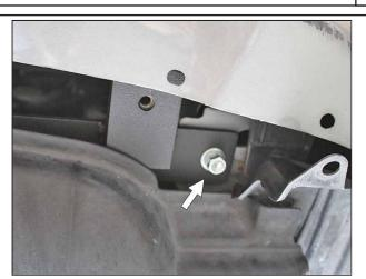
Attach the mounting brace to the lower bumper beam by using (1) 3/8 washer, (1) 3/8 lock washer, (1) 3/8 nut.
