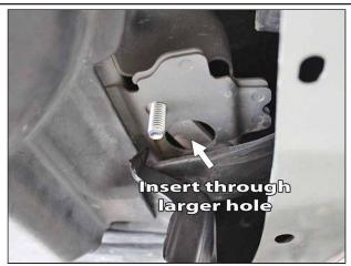
Locate the two holes in the lower bumper beam, and insert the bolt plates.
