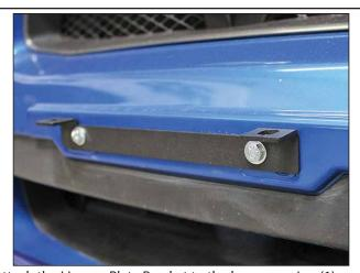
Attach the License Plate Bracket to the bumper using (1) 1/4" Lag Screw and (1) 1/4" Flat Washer in each mounting hole to the factory location. Note: Loosely fit to allow adjustment.
