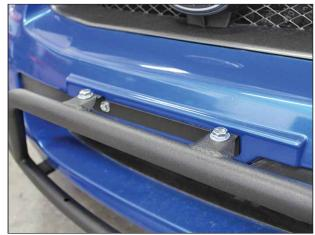
Attach the light bar to License Plate Bracket using (1) 3/8"-16x 1" hex bolt, (2) flat washer, (1) lock washer, and (1) 3/8" nut for each side.
