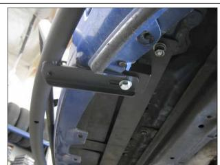
Attach the light bar to the lower brace using (1) 3/8"-16x 1", (1) 3/8" Lock Washer, and (1) 3/8" Flat Washer on each side. Tighten all 3/8" hardware to 33 ft-lbs.
