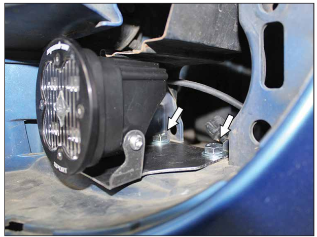
Insert (1) 5/16"-18 x 1" Hex Bolt and (1) 5/16" Flat Washer into each slot on the mounting bracket and fasten to the vehicle using (1) 5/16" Flat Washer, (1) 5/16" Lock Washer and (1) 5/16"-18 Hex Nut on the bottom side.
