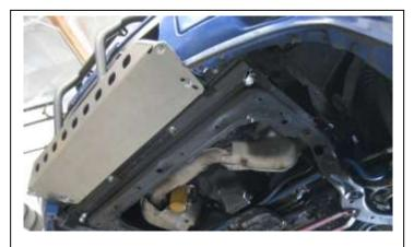
With the ultimate light bar hanging, attach the bottom of the aluminum skid guard to the lower brackets using (1) 3/8"-16 x 1" hex bolt, (2) 3/8 washer, (1) 3/8 lock washer, (1) 3/8 nut. Tighten all 3/8 hex bolt to 32 ft-lb. Tighten all M8 Bolt to 25 N-m (19 ft-lb).
