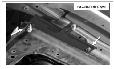
Attach the mounting bracket to the car using the factory bolt, and (1) 3/8" flat washer in the forward location. Attach the rear tab using (1) 3/8"-16x1 ¾" hex bolt, (2) 3/8 flat washer, (1) nylon spacer, (1) 3/8 lock washer, and (1) 3/8 nut.
