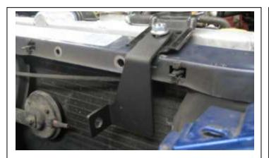
Attach the upper brackets by removing the radiator support screw.
