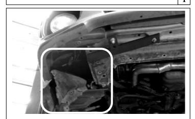
**Note:** Factory splash guards may need to be partially removed to gain access to the mounting point on the lower sub-frame.
