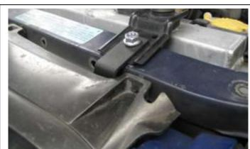
Attach the grille back on and insure all the clips are fastened.
