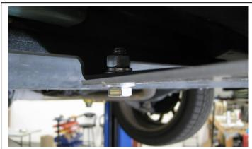
Mount the Skid Guard to the lower brackets using (1) 3/8"-16x1" hex bolt, (2) 3/8" flat washer, (1) 3/8" lock washer, and (1) 3/8"-16 nut.
