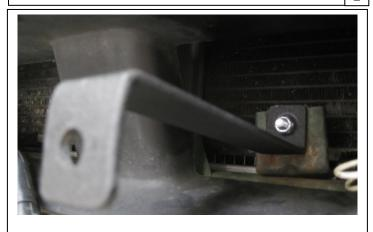
Mount the the Z-bracket to the lower radiator support using (1) 1/4"-20 x 3/4" hex bolt, and (1) 1/4"-20 nyloc jam nut.
