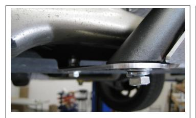
Mount the Skid Guard to the upper bar using (1) 3/8"-16x ¾" hex bolt, (1) 3/8 flat washer, and (1) 3/8" lock washer.
