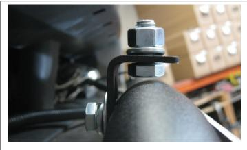
Attach the L-bracket to the upper bar using (1) 5/16"- $18 \times 1$ " hex bolt, (1) 5/16" flat washer, and (1) 5/16" lock washer. Insert (1) 3/8"- $16 \times 3$ 4" hex bolt, (1) 3/8" lock washer, and (1) 3/8"- $16 \times 3$ 10 nut into the hole of the L-bracket.
