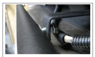
Attach the upper bar of the Skid Guard to the Z-bracket using (1) 5/16"-18x1" hex bolt, (1) 5/16" flat washer, and (1) 5/16" lock washer.
